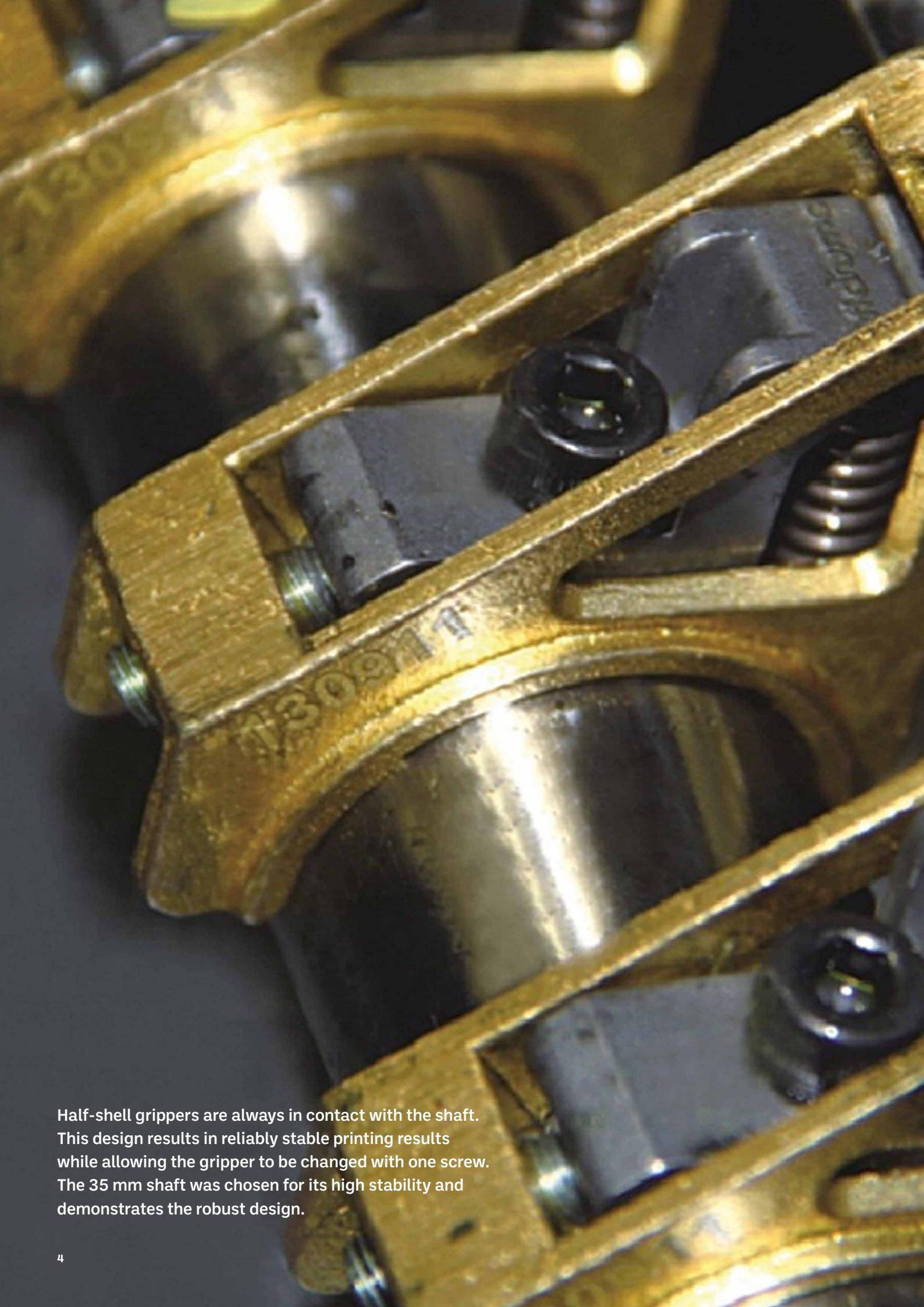
Half-shell grippers are always in contact with the shaft.
